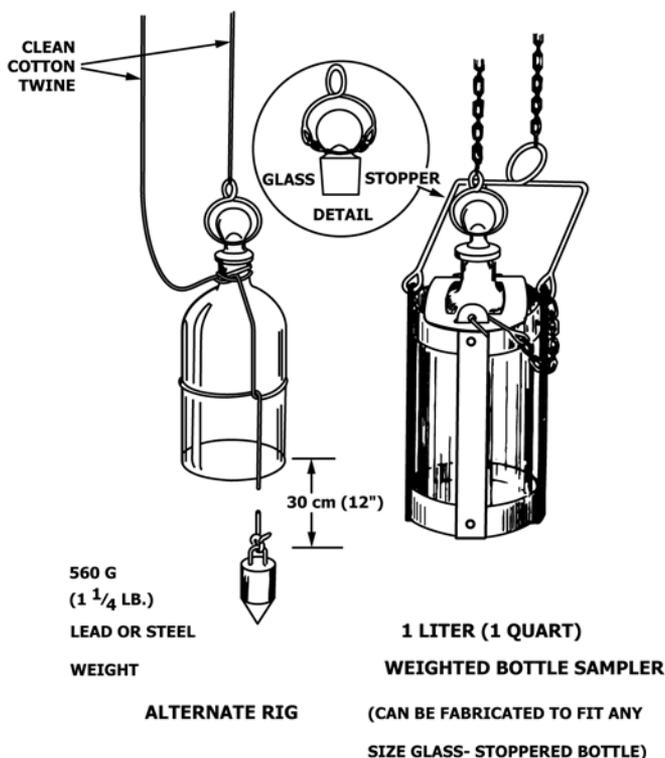
FIG. 2 Assembly for Bottle Sampling
