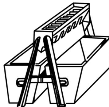
FIG. 21 Riffle Sampler
