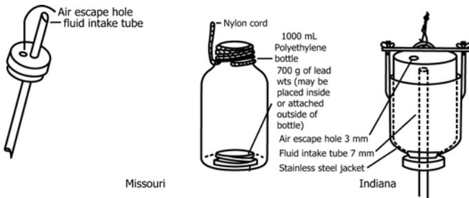
FIG. 24 Missouri and Indiana Weighted Restricted-Fill Fluid Fertilizer Sampling Bottles Designed to Fill While Being Lowered (and Raised) in Storage Tanks
