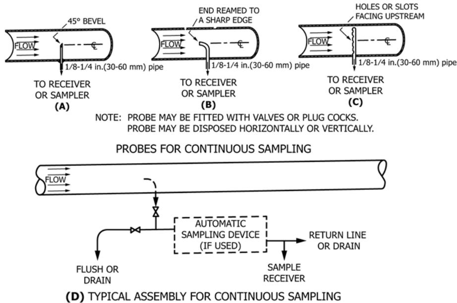
FIG. 5 Probes for Continuous Sampling
