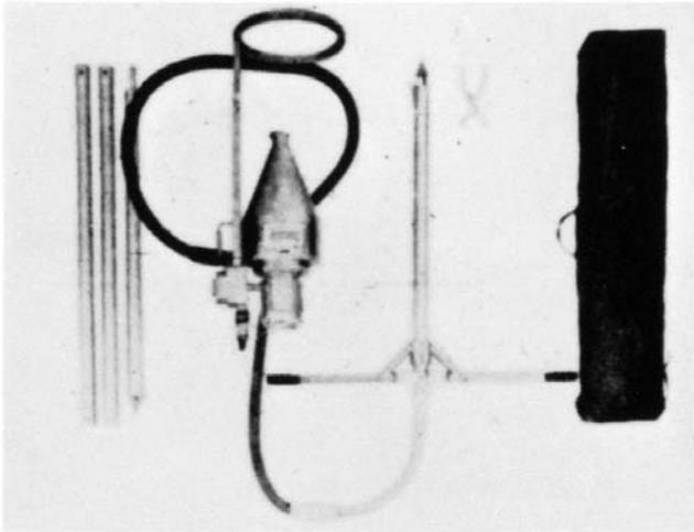
FIG. 15 Vacuum Sampler
