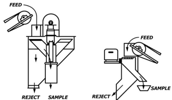
FIG. 17 Falling-Stream Samplers
