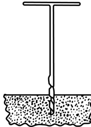
FIG. 14 Auger Sampler
