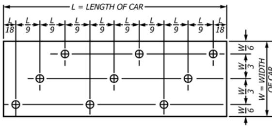
FIG. 19 Location of Sampling Points from the Exposed Surface of the Car
