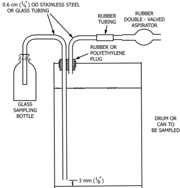
FIG. 7 Alternative Tube Sampling Assembly
